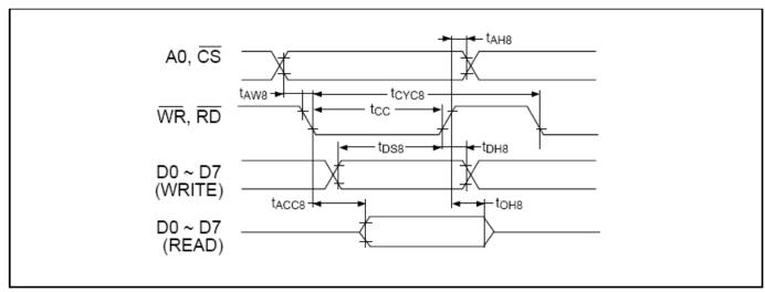
$Ta = -0 \text{ to } 50^{\circ}\text{C}, \text{ VSS} = -5.0\text{V} \pm 10\%, \text{ Unit: ns}$
